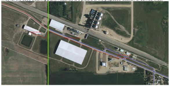
Sewer would be a pumped from existing septic tank & terminated in the existing sanitary manhole for serviceability. Lines would be directionally drilled to minimize disturbance. Curb stops would be located at properly line. Client would be responsible for all costs of installation & materials.
